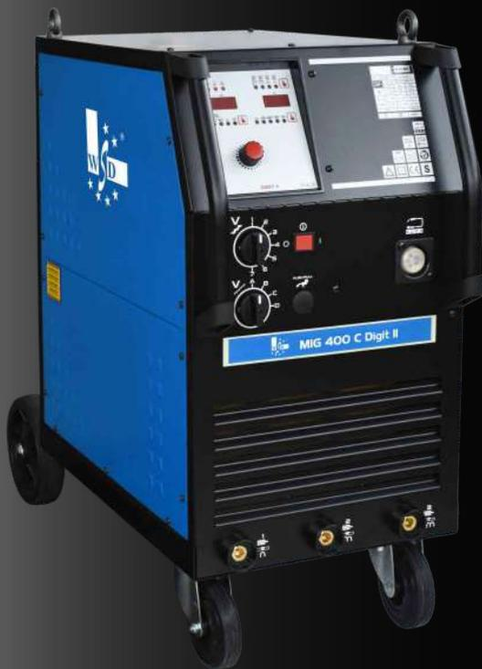
• Three phased MIG/MAG welding machines, step controlled, with integrated wire feeder. Primary and secondary parameters visible on 2 displays with welding current and welding voltage simultaneous reading. Allows welding of all steel types all stainless steel, aluminium and copper alloys and fluxed core wires. Suitable for medium and heavy metal construction, repair shops and naval shipyards.
